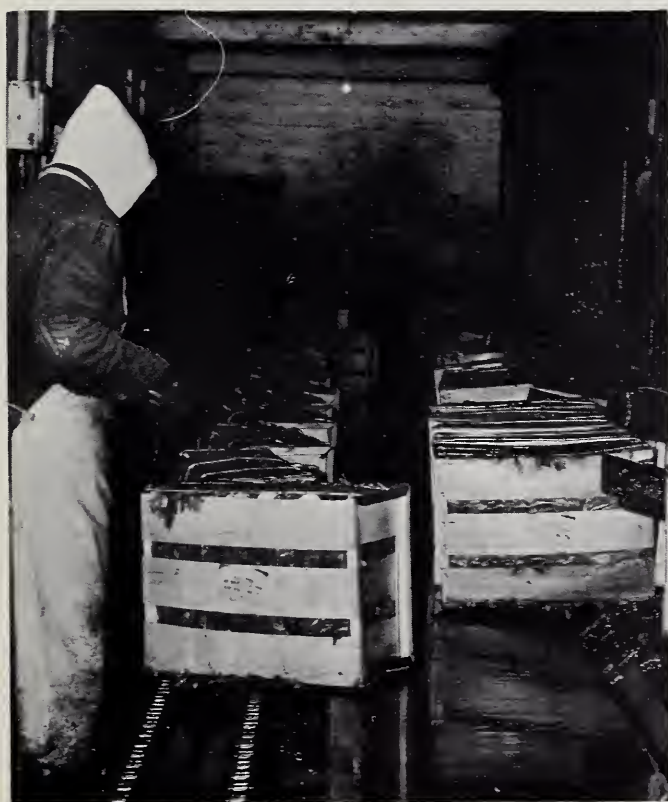
Figure 4.--Pulling crates of celery from the hydro-cooling tunnel onto a chain conveyor.
